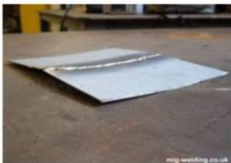
Figure: Distortion in Sheet due to Welding
