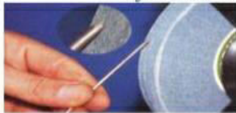
Figure 17-Correct method of grinding a tungsten electrode.
