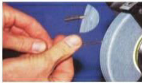
Figure 16 - Incorrect method of grinding a tungsten electrode
